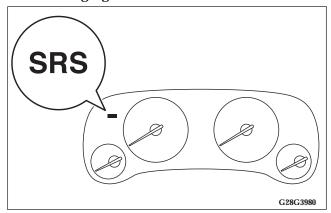
There is a Supplemental Restraint System (SRS) warning light on the instrument panel. The system checks itself each time the ignition is turned on and the light indicates if there is a problem.
